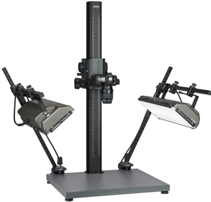
For classic reproduction work, it is important to light the originals homogeneously and with equal light intensity by using two Copy Ones, one to the left and one to the right of the original and set at the same angle (typically 45°). We recommend the use of a light meter with a flat calotte to check lighting and light intensity.
